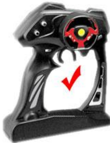
5. Release the trigger to neutral
