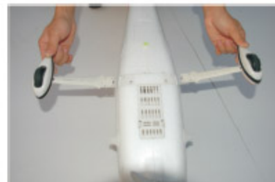
3. Install the main landing gear.
