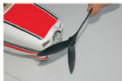
10. Install the propeller.
