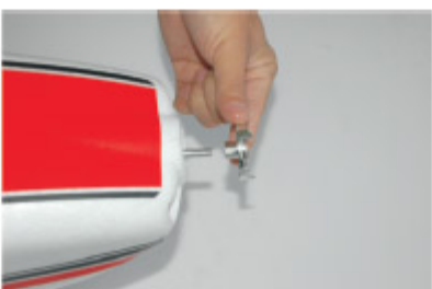
9. Install the back plate of the spinner.
