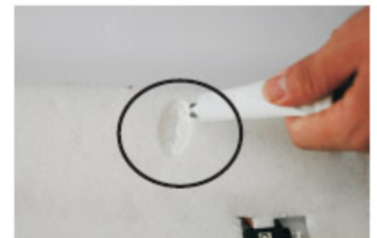
18. Apply glue in the slot of the main wing.
