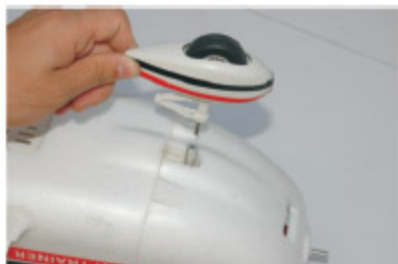
1. Install the front landing gear.
