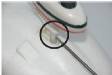
2. Secure the front landing gear.
