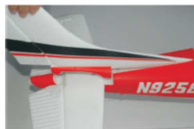
8. Install the rudder.
