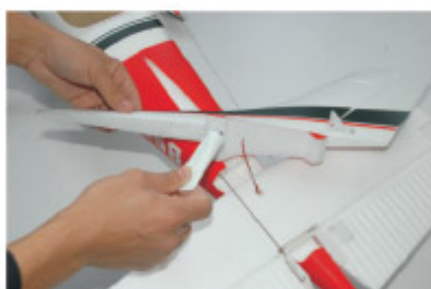
7. Apply the glue on the combined side of the rudder.
