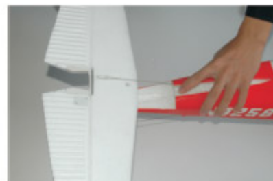
5. Install the elevator.
