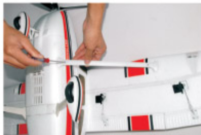
20. Install the supporting bar Screw PM3.0X8(4PCS)
