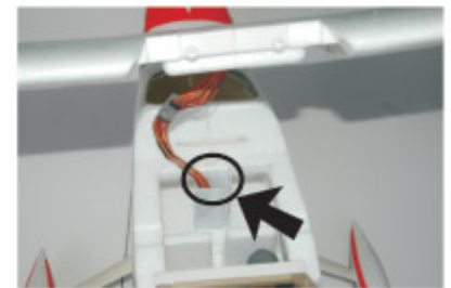
16. Insert the wires into the hole.
