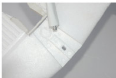
4. Apply glue on the combined side of the elevator.
