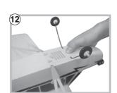
gear slot, and tighten by forcing down the landing gear cover.
