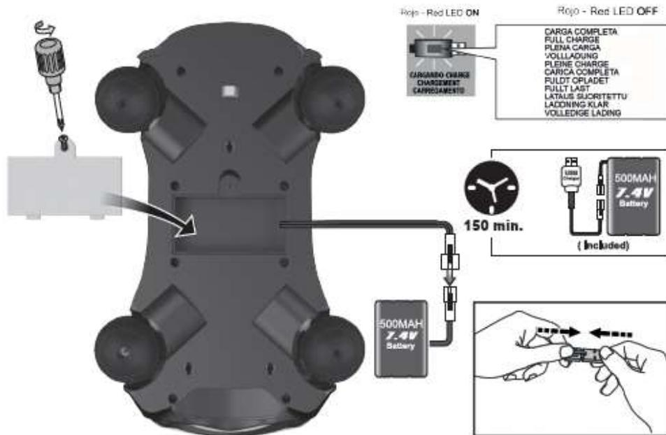
VIGILAR PROCESO DE CARGA - KEEP AN EYE ON CHARGING PROCESS - MONITORAR O CARGAMENTO - ACHTEN SIE AUF DEN LADEVORGANG - IL FAUT SURVEILLER LA CHARGE - SORVEGLIANZA DI LA CARICA - OVERVÅK LA DEPROSESSEN - VALVU LATAUSTA - ÖVERVÅKA LADDNINGSPROCESSEN - MONITOR LAADPROCES
